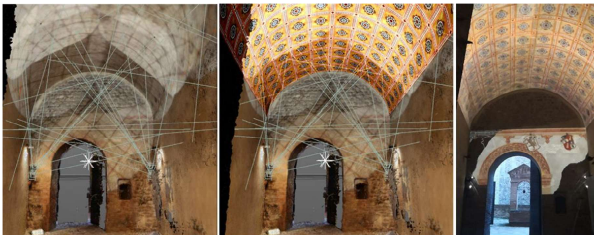
Figure 9. The sequence of geometric operations carried out to determine the definitive projection. Left to right: 3d digital model with cameras placed in the projection points; 3d model mapped with reconstructed texture of lacunars; picture of the final projection on the real vault
